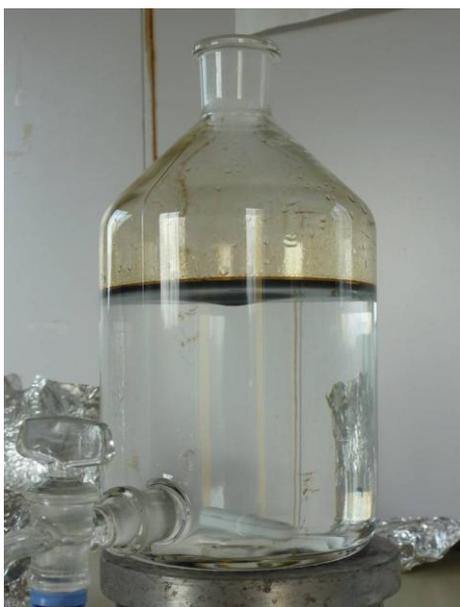
Figure 2: Preparation of an oil WAF
