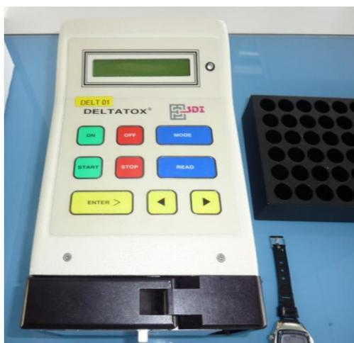
Figure 3: Delta Tox field instrument
